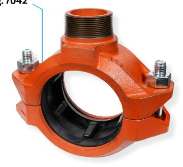
The Gruvlok Fig. 7042 Outlet Coupling is designed to join two sections of grooved end pipe and form a reducing outlet connection. The outlet couplings are available for the  $1\frac{1}{2}$ " through 6" IPS or ISO run pipe sizes with the outlet pipe sizes ranging from  $\frac{1}{2}$ " through 2".
